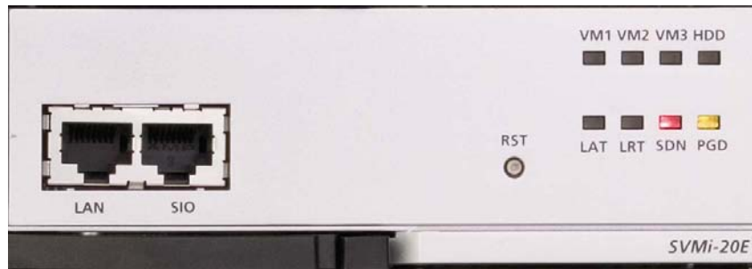
Figure 3.42 SVMi-20E LED Indications
